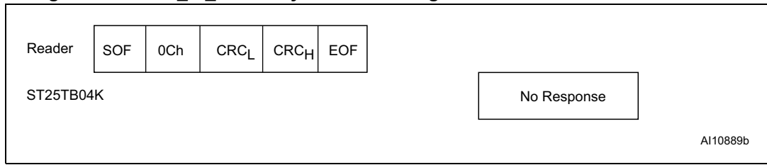
Figure 53. Read_block frame exchange between reader and ST25TB04K
