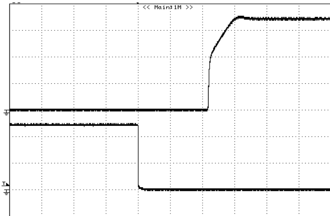
Figure 19: Turn on delay time at remote on 7Vin, 0.69V/12A out. (Top: VOUT, 0.2V/div; Bottom: ON/OFF, 2V/div; 2mS/div)
