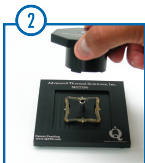
Position the Knob Tool over the Frame Clip
