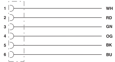
Contact assignment of 7/8" socket
