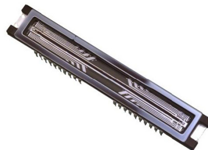
Figure 1. KLI-8023 Linear CCD Image Sensor
