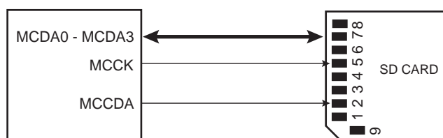
Figure 33-6. SD Card Bus Connections with One Slot
