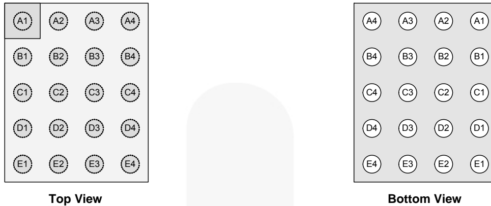
Figure 4. WLCSP-20 Pin Assignments
