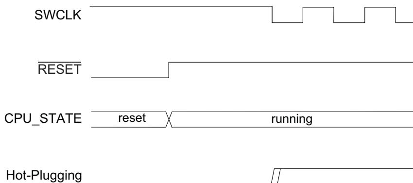
Figure 12-3. Hot-Plugging Detection Timing Diagram
