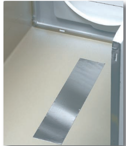
3M™ Damping Foil 2552 on the inside of a washing machine reduces structure-borne noise and reduces vibrational fatigue to decrease the risk of part loosening and displacement.
