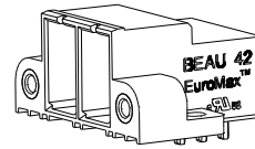
2 AND 3 CIRCUIT HEADERS HAVE NO "PRY SLOTS"
