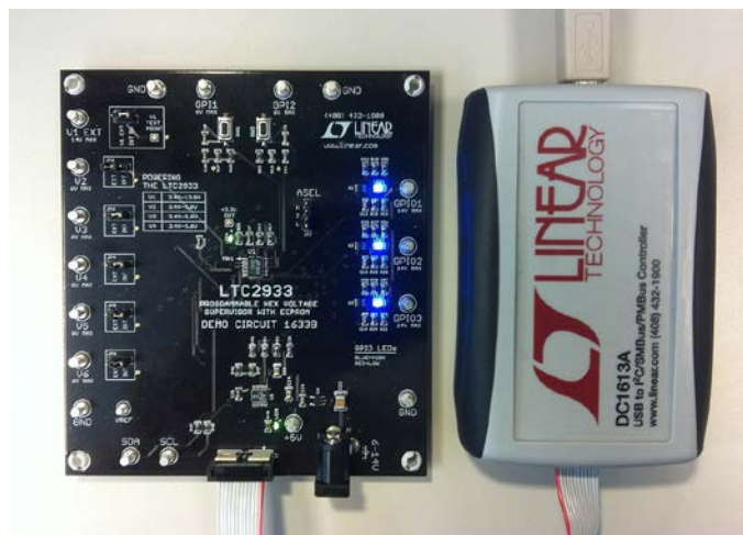
Figure 4. Connecting DC1633B Board and the DC1613 USB to I 2 C/SMBus/PMBus Controller
