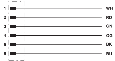
Contact assignment of 7/8" plug
