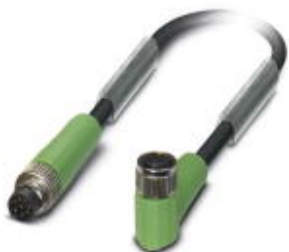
Sensor/actuator cable, 8-position, PUR halogen-free, black RAL 9005, Plug straight M8, on Socket angled M8, cable length: 0.3 m
