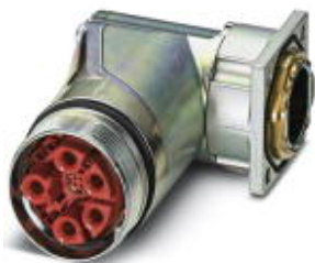
Device connector for front wall, angled rotatable, shielded: yes, SPEEDCON, M40, type of contact: Socket, Crimp connection, Axial O-ring, 4x Ø4,2
