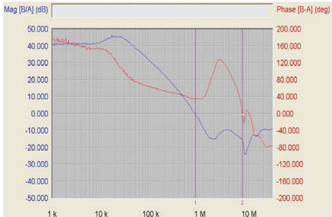
Figure 2 — Gain and Phase Bode Plot Fc = 810KHz, PM = 36 degree at 1A Source
