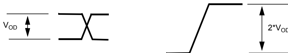
Figure 21 - Differential Voltage Definition
