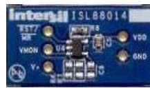
FIGURE 22. THE TYPICAL ISL8801XEVAL1Z MEASURING 0.5" x 1"
