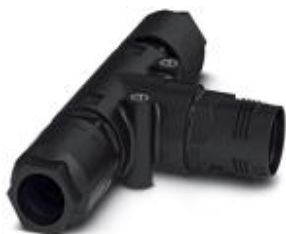
QUICKON T-distributor, black, 4+PE-pos., 2.5 mm 2 ... 6.0 mm 2 /690 V/40 A, for cable diameter of 9 mm ... 14 mm, with two QUICKON nuts
