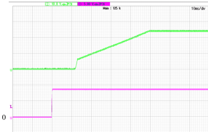
Turn-on transient at full load current (10ms/div). Top Trace: Vout; 10V/div; Bottom Trace: ON/OFF input: 5V/div.
