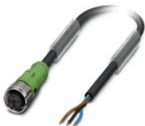
Sensor/actuator cable, 3-position, Variable cable type, free cable end, on Socket straight M12 SPEEDCON, A-coded, PIN 2+4 bridged, cable length: Free input (0.2 ... 40.0 m)
