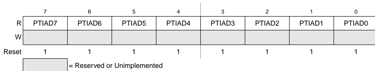
Figure 2-20. Port AD Input Register (PTIAD)
