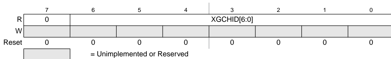
Figure 5-4. XGATE Channel ID Register (XGCHID)
