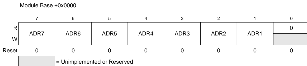
Figure 13-3. IIC Bus Address Register (IBAD)
