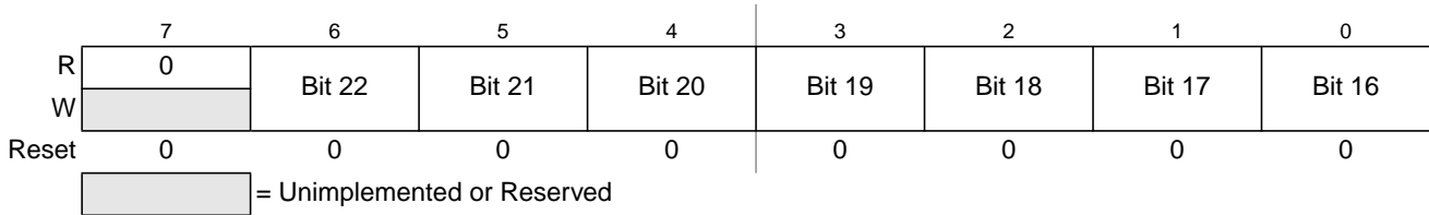
Figure 22-15. Debug Comparator Address High Register (DBGXAH)
