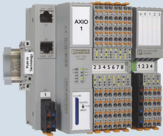
I/O system and controller with push-in connection
