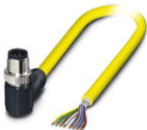
Sensor/Actuator cable, 8-position, PVC, yellow, shielded, Plug angled M12 SPEEDCON, A-coded, on free cable end, Cable length: 10 m
