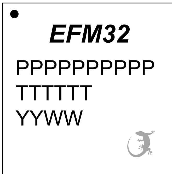
Figure 10.3. TQFP48 Package Marking
