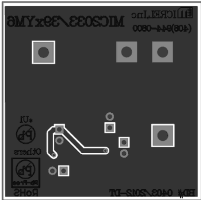
MIC2033-xxxYM6 Evaluation Board – Bottom Layer
