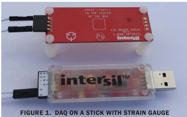
FIGURE 1. DAQ ON A STICK WITH STRAIN GAUGE
