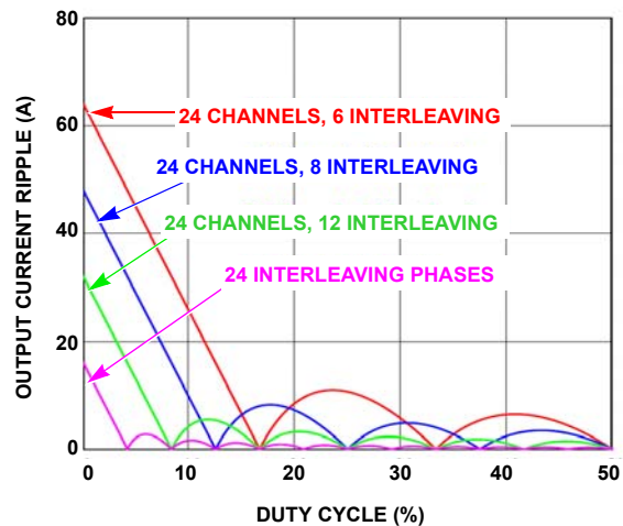
FIGURE 13. OUTPUT CURRENT RIPPLE vs DUTY CYCLE, PHASE COUNT
