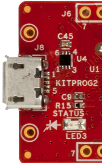
Figure A-8. USB 2.0 Micro-B connector J8
