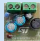
STEVAL-ISA178V1 5 V/200 mA buck-converter based on VIPer01
