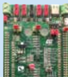
STEVAL-CCC001 STUSB1600A USB Type-C evaluation board
