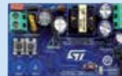
STEVAL-ISA192V1 7 W not-isolated flyback with smart standby using VIPerOP and touch sensing
