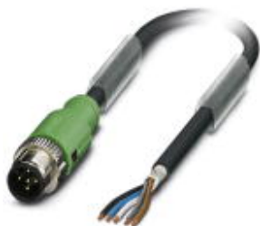
Sensor/actuator cable, 5-position, PUR halogen-free, black-gray RAL 7021, shielded, Plug straight M12 SPEEDCON, A-coded, on free cable end, cable length: 3 m
