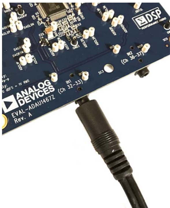
Figure 12. Analog Stereo Input Source Connection
