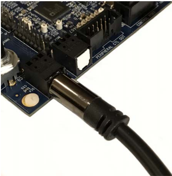
Figure 35. Photograph of the Optical S/PDIF Input Connection
