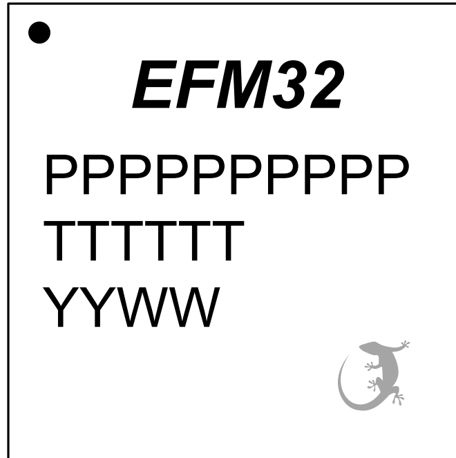
Figure 8.3. QFN48 Package Marking
