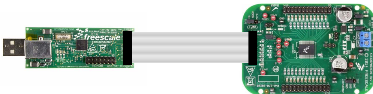
Figure 6. Connecting KITUSBSPIDGLEVME to the Evaluation Board
