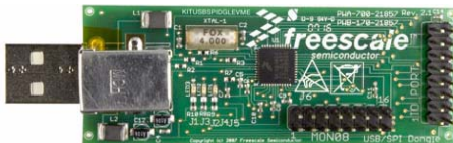
Figure 5. KITUSBSPIDGLEVME Interface Dongle
