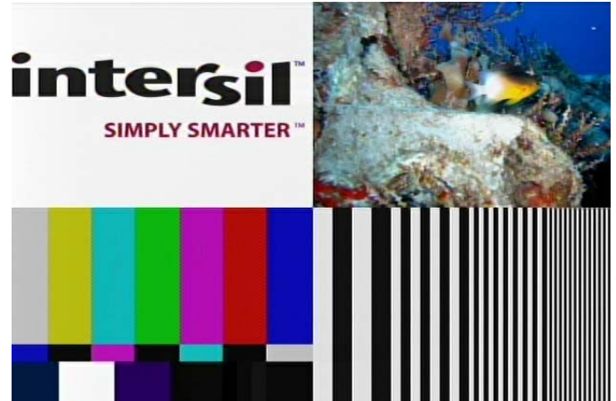
FIGURE 6. TEST PATTERN IMAGE AFTER 2000 FEET OF CAT 5 WITH ISL59602 (OR BETTER)
