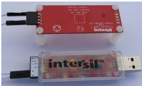
FIGURE 1. DAQ ON A STICK WITH STRAIN GAUGE
