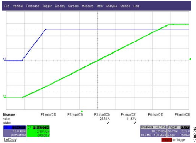
Figure 16. Startup at 350 VDC, 25 A Load (1 A/ \mu s Slew Rate) Green Trace: Output Voltage, 2 V/div, 10 ms/div Blue Trace: Load Current, 10 A/div, 10 ms/div
