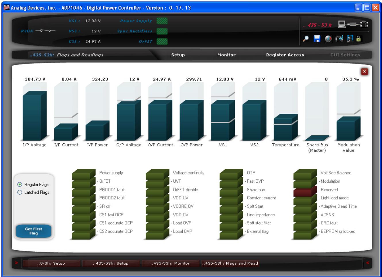
Figure 11. Flags and Readings Window in GUI Showing the Entire Status of the PSU at Full Load
