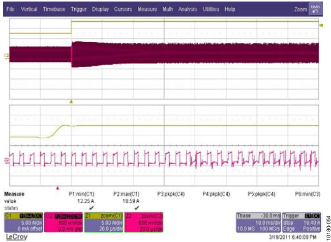
Figure 55. Input Current During Load Step of 10 A to 20 A Yellow Trace: Load Current, 5 A/div, 10 ms/div Red Trace: Voltage at CS1 Pin, 500 mV/div (20 \mu s/div Zoomed In)
