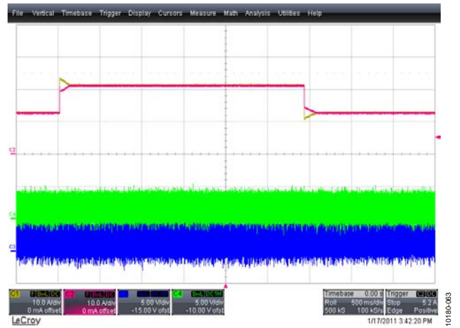
Figure 64. Digital Current Sharing with Load Step of 25 A, 42 A, 25 A Red and Yellow Traces: Output Currents of PSU1 and PSU2, 10 A/div, 500 ms/div Green and Blue Traces: SHAREo Pins of PSU1 and PSU2, 5 V/div, 20 ms/div
