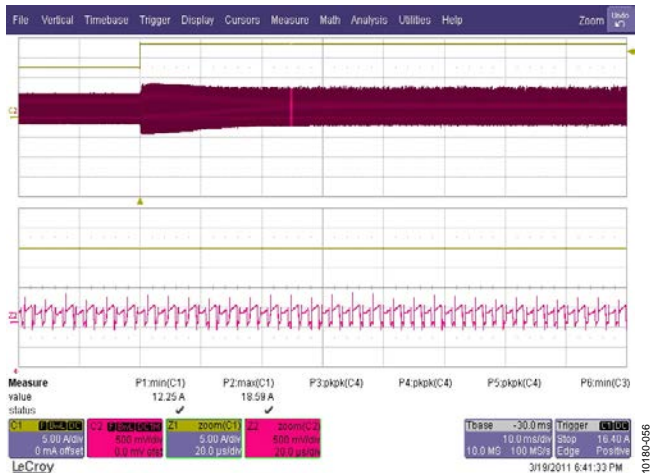
Figure 57. Input Current During Load Step of 10 A to 20 A Showing Steady Balancing of Both Phases; Yellow Trace: Load Current, 5 A/div, 10 ms/div Red Trace: Voltage at CS1 Pin, 500 mV/div (20 \mu s/div Zoomed In)
