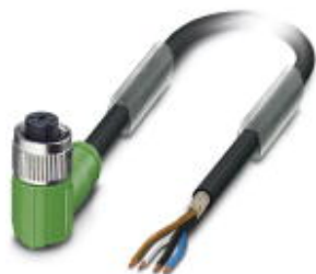
Sensor/actuator cable, 4-position, Variable cable type, shielded, free cable end, on Socket angled M12, A-coded, cable length: Free input (0.2 ... 40.0 m)
