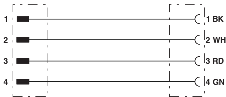
Contact assignment of 7/8" plugs/sockets
