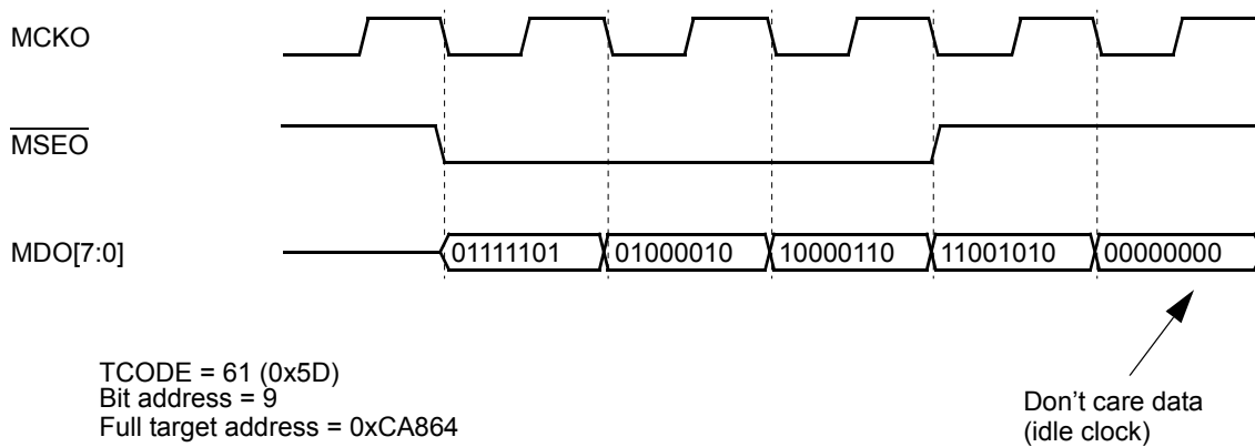
Figure 24-43. Indirect Branch Synchronization Message with Compressed Code
