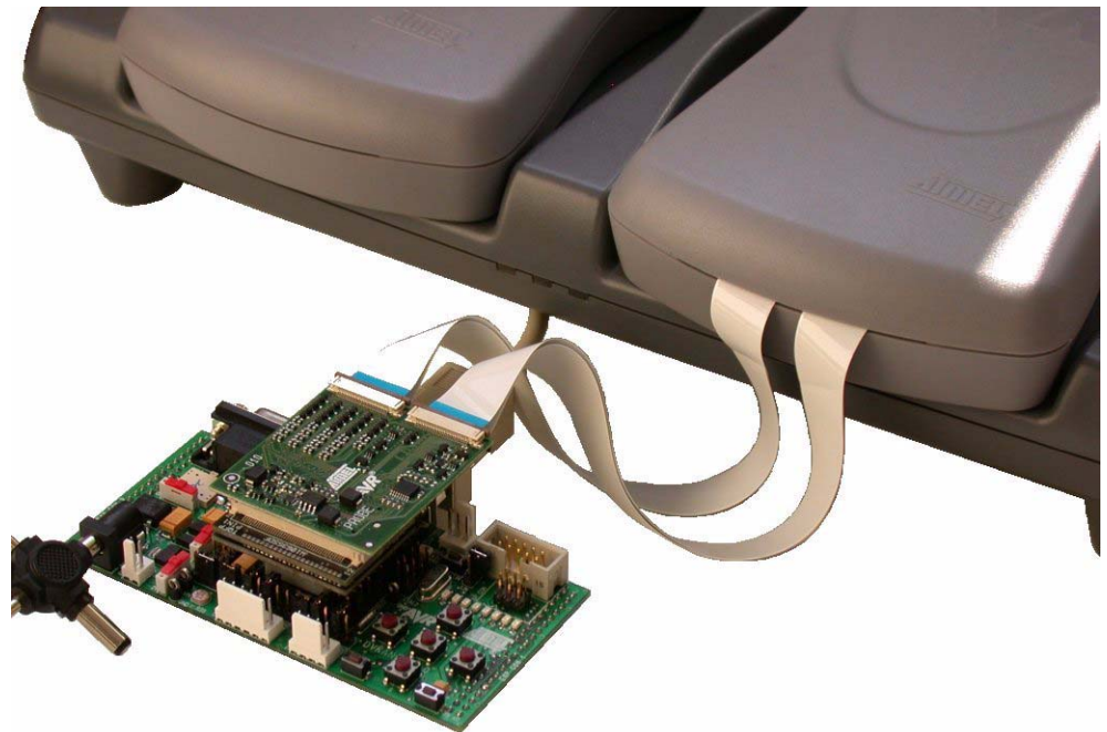
Figure 3-46 . Connecting AVR ICE 50 for Debugging
