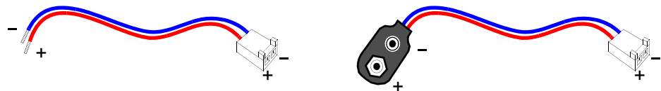
Figure 3-5 . EXT PWR Female Connector / Cable for 9V Battery
