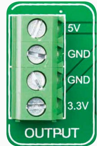
Figure 20-1: Output voltage terminals
