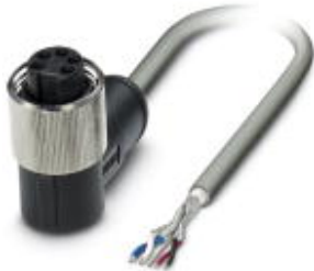
Bus system cable, DeviceNet, 5-position, PUR halogen-free, Gray RAL 7001, Free cable end, on Socket angled 7/8"-16UNF, Cable length: 15 m
