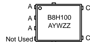
SO-8 FLAT LEAD CASE 488AA STYLE 2
