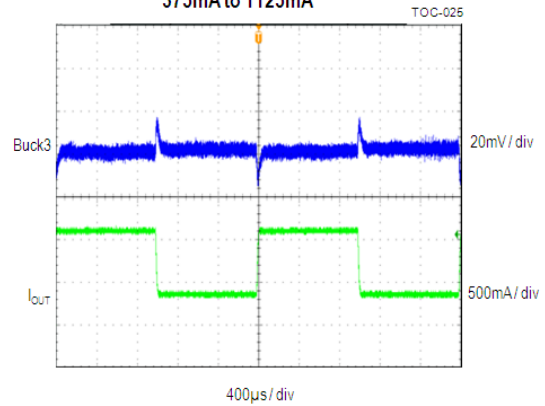
Load Transient LDO2-Vout=1.8V 37.5mA to 112.5mA
