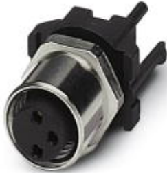
Sensor/actuator flush-type socket, 3-pos., M8, rear/screw mounting with M8 thread, polarity protection, with straight solder connection, model with 6 mm long terminal pins
