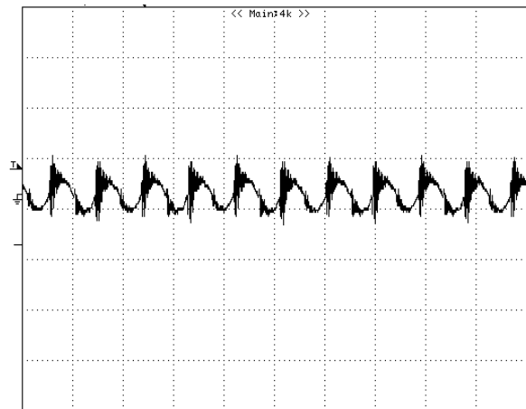
Figure 11: Input Terminal Ripple Current, i_c , at full rated output current and nominal input voltage with 12\mu H source impedance and 33\mu F electrolytic capacitor (200 mA/div, 2us/div).
