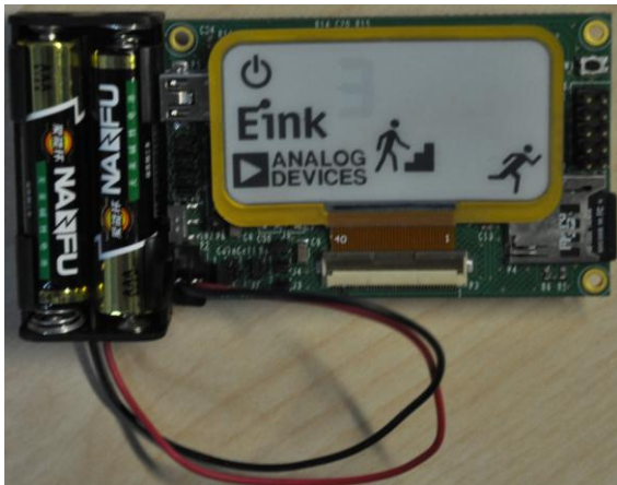
Figure 40. Data Logger with Portable Supply
