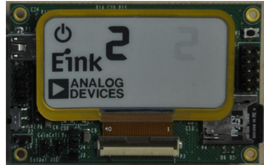
Figure 31. E-ink Display for Second Inactivity Interrupt
