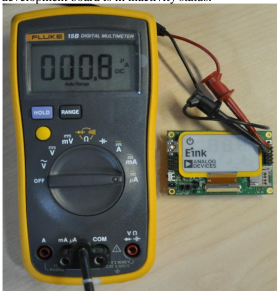
Figure 26. EVAL-ADXL362Z-DB in Inactivity Status
